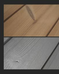
Thermally modified products are natural, free of chemicals, with a long service life and can be recycled. Thermal modification is a method in which only heat and steam is used.
